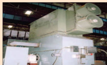
Slow Speed Pressurised Sy. Motor (1.2 MW, 6.6 KV, 18P For IOCL, Mathura)
