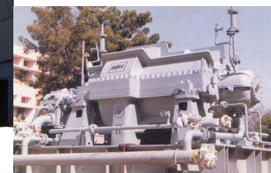
Fabricated Compressor for inert gas application
