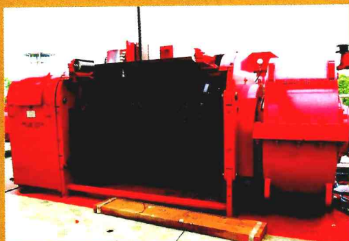
AC VFD DRAW WORKS
