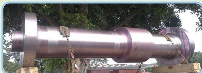
Hydro Turbine Shaft
