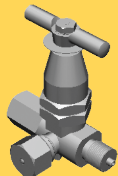
Pressure Gauge Valve
